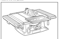
2. Position the rip fence to the desired width of rip and lock in place by pivoting the grip. Before ripping, make sure the rear end of the rip fence is secured firmly. If it is not secured enough, follow the procedures in the section titled "Installing and adjusting rip fence".
