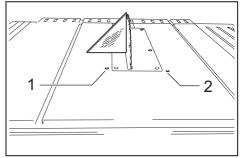
▶ 1. 90°Adjusting screw 2. 45°Adjusting screw
