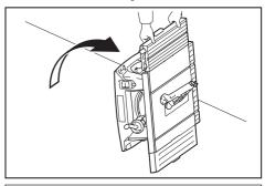
ACAUTION: Be sure to support the tool so as not to let the tool fall down. It is recommended to have someone to support the tool.
