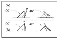
The tool is equipped with positive stops at 90° and 45° to the table surface. To check and adjust the positive stops, proceed as follows:
