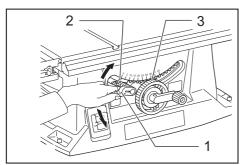
■ 1. Lock lever 2. Arrow pointer 3. Handwheel
