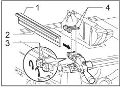
▶ 1. Rip fence 2. Groove 3. Nut 4. Screw head
