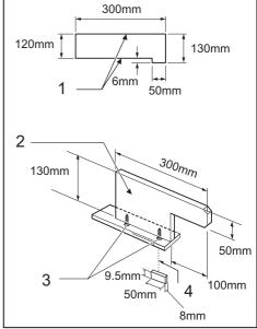
▶ 1. Face/edge parallel 2. Handle 3. Wood screw 4. Glue together
