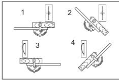
1. Cross cutting 2. Mitering 3. Bevel cutting
