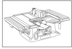
When the width of rip is 65 mm - 150 mm wide, use the push stick to feed the workpiece.
