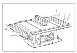
Make sure that the tool is unplugged. Carry the tool by holding the tool part shown in the figure.
