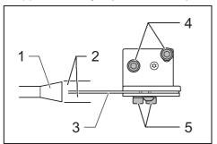
1. Saw blade 2. These two clearances should be equal. 3. Riving knife 4. Hex bolts (B) 5. Hex bolts (A)
