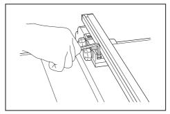
**ACAUTION:** Be sure to adjust the rip fence so that it is parallel with the saw blade, or a dangerous kickback condition may occur.
