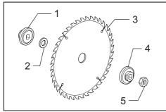
Inner flange 2. Ring 3. Saw blade 4. Outer flange
