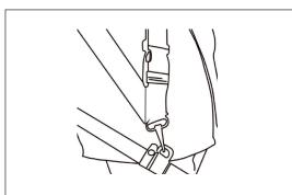
Press the both side of the release button with one hand, the machine can be released quickly from the operator in the event of emergency (e.g. occur spark, smoking or vibrate abnormally).
