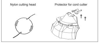
CAUTION: The appropriate protectors must always be installed for your own safety and in order to comply with accident-prevention regulations. Operation of the equipment without the guard installed is prohibited.
