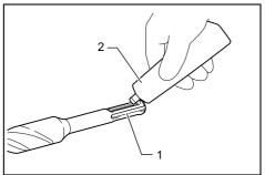
Shank end of the drill bit/chisel 2. Grease
