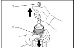
▶ 1. Drill bit/chisel 2. Chuck cover
