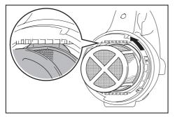
Install the capsule. Align the mark on the capsule with the mark near the handle and then firmly twist the capsule in direction of the arrow until it is secured.
