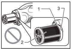
1. Groove of cleaner housing 2. Prefilter 3. Securing lip
