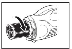
Connect capsule. Align O symbol on capsule with O symbol on handle and then firmly twist capsule in direction of arrow until it is secured.
