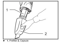
Twist prefilter in direction of arrow to unfasten securing lip from cleaner unit and then pull off prefilter.
