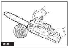
2. With the saw chain running, saw into the wood while using the rear handle to raise the saw and the front one to guide it. Use the spike bumper as a pivot.
