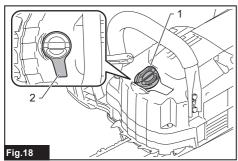
▶ 1. Oil tank cap 2. Oil inspection window
