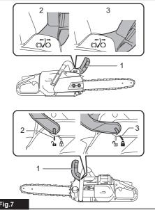
1. Front hand guard 2. Unlocked position 3. Locked position
