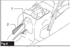
■ 1. Switch trigger 2. Lock-off lever
