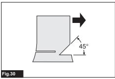
**NOTE:** The scarf determines the direction in which the tree will fall, and guides it. It is made on the side towards which the tree is to fall.
