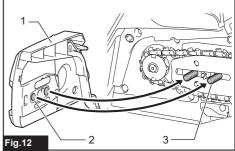
1. Sprocket cover 2. Hole 3. Bolt
