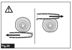
When you cut a wood under tension, cut the pressured side (A) first. Then make the final cut from the tensioned side (B). This prevents the bar from becoming trapped.
